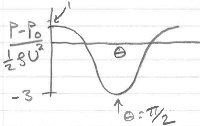
We can use this to calculate the drag ( $F_x$ ) on the cylinder!
