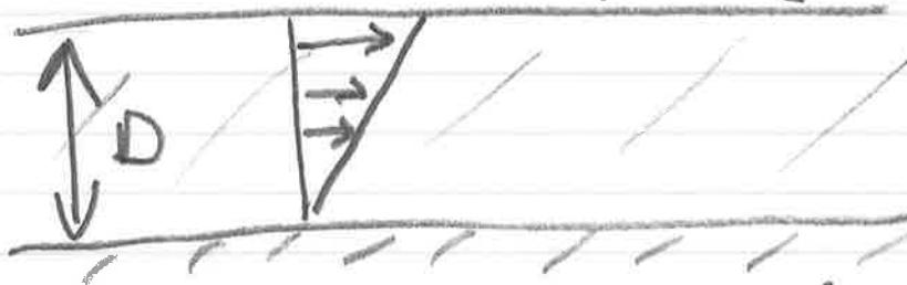
If mat'l is elastic solid, we get some fixed displacement  $\Delta x$  for a given force  $F$  at S.S.
