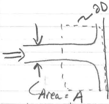
Water velocity in this frame is now  $(\underline{u_j} - \underline{u})$ , not  $\underline{u_j}$ !
