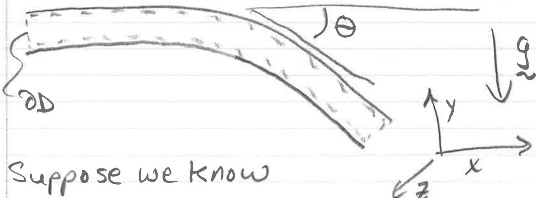
Suppose we know inlet & outlet pressures as well as the flow rate. We want to know the force exerted by the fluid on the bend (section of pipe) which is ( $\rightarrow$ ) force exerted by bend on fluid!
