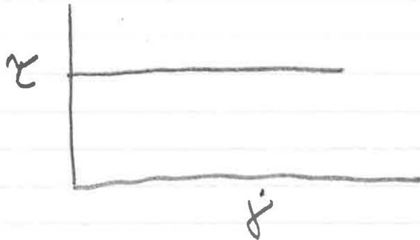
indeterminate shear rate for applied shear stress! Leads to complex patterns in cytological streaming!
