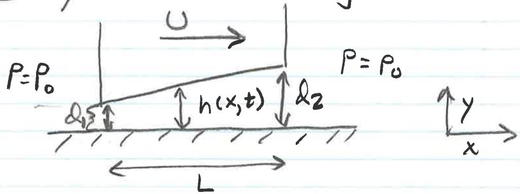
If  $H \equiv d_1 \ll L$  we can use lubrication theory to calculate the upward force on the block for some  $U, d_1, d_2, L$ , etc.
