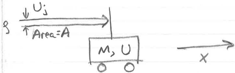
A jet of water of diameter  $D$  & velocity  $U_j$  impinges on the plate. What is the force on the plate as a function of  $U$ ? What is the velocity of the car as a function of time?
