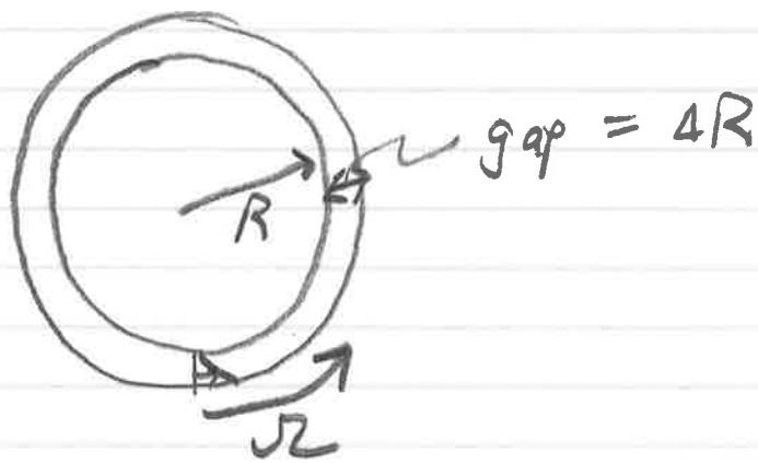
By rotating the outer cylinder you deform the fluid in the gap and exert a torque on the inner cylinder. This torque is used to calculate the viscosity!
