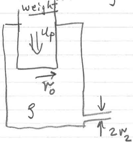
For a given motion of the piston, what is the flow rate thru the outlet pipe? For a given weight of car, what is the pressure in the pipe?
