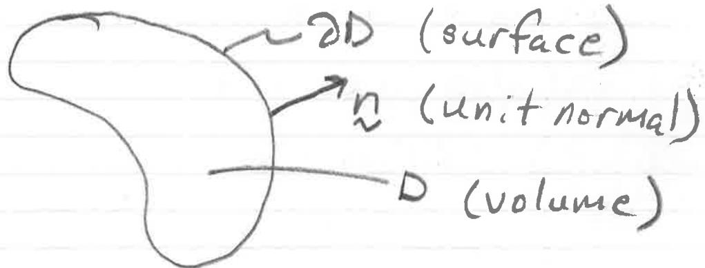
What are the forces on the molecules in  $D$ ? Divide into Surface Forces and Body Forces!
