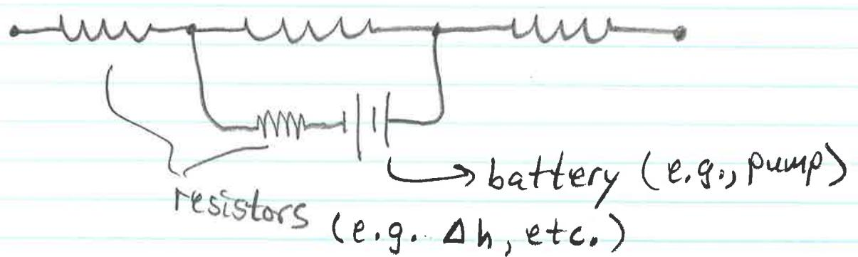
The head is equivalent to the voltage. The flow rate is equivalent to the current. The only difference is that
