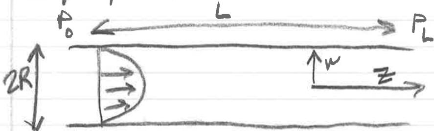
Suppose we have an axial pressure gradient (e.g.,  $\frac{\partial P}{\partial z} \neq 0$ )
