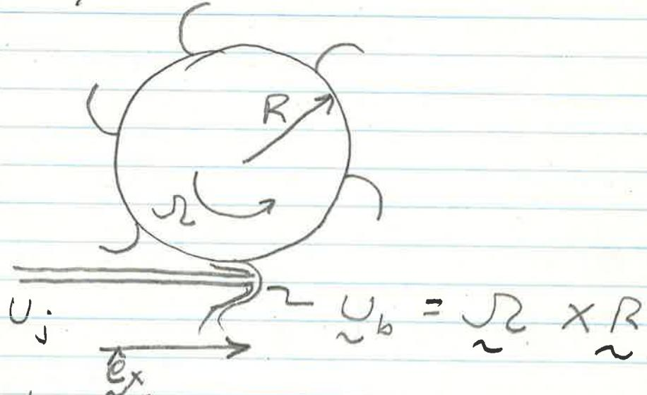
We wish to determine the torque on the wheel, and the rate of work (Power) transferred to it!
