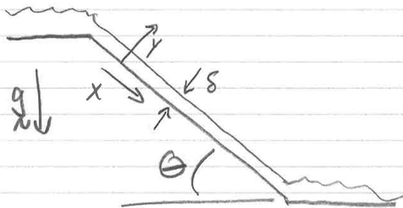
IF the fluid is viscous, it will rapidly reach some constant thickness  $s$ , and some steady velocity profile. What is the relationship between  $Q/W$ ,  $u$ ,  $s$ ,  $\beta$ ,  $\mu$ ,  $g$ , and  $\theta$ ? Just apply the Navier-Stokes equations!
