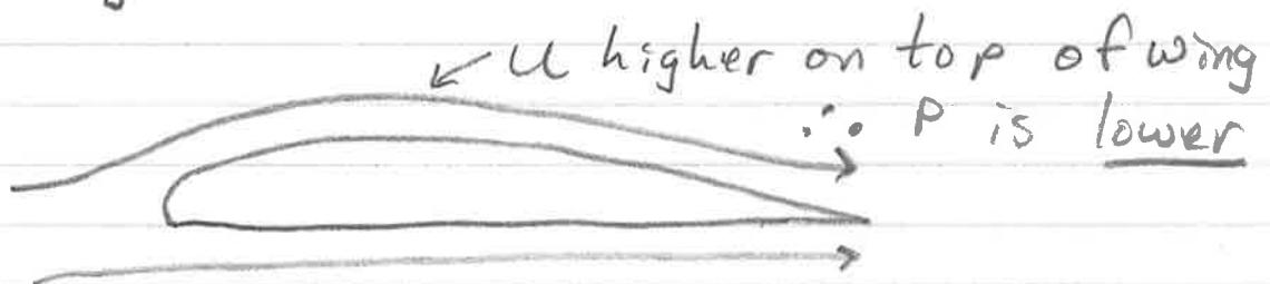
The  $\Delta P$  from top to bottom provides Lift which makes the plane fly!
