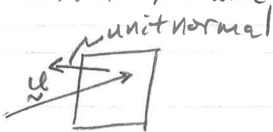
Volumetric flux  $\equiv \frac{\tilde{u}}{A} \Rightarrow \frac{\text{Vol}}{\text{Area} \cdot \text{Time}}$
