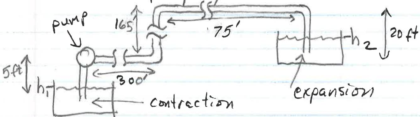
Suppose we have all 4" ID smooth pipe, and we want a flow rate  $Q = 42 \text{ ft}^3/\text{min}$ .
