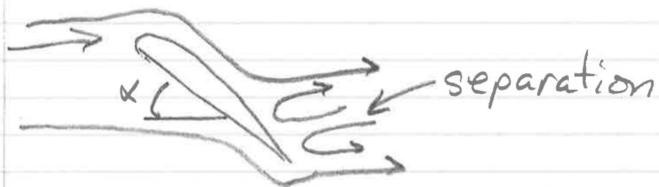
Separation does two things. First, it greatly increases drag, decreasing the L/D ratio and, since engines aren't designed to overcome this force, the plane slows down! Since  $L \propto gV^2$ , slowing down the plane kills the lift, and the plane falls! Second, wing control surfaces (e.g. elevators) are on the trailing edge of the wing. If the
