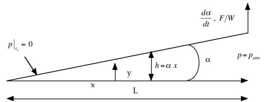
Two plates of length L in contact at one edge are separated by a very small angle  $\alpha$ . For small angles the gap between the plates is given by  $h = \alpha x$ , where x is the distance from the vertex. The plates are pulled apart at some rate  $d\alpha/dt$ .
